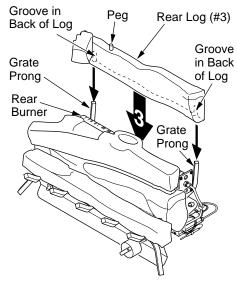
Figure 23 - Installing Rear Log (#3) [18" Variable Manually-Controlled Set Shown]
